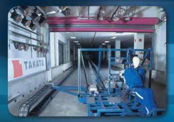
Very high stresses are transmitted to the cable drag chain system in necessary crash tests. Acceptable service life can only be achieved with the system with the most stable system components.
