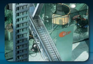
Murrplastik Systemtechnik GmbH, based in Oppenweiler, developed technically unparalleled cable drag chains for a globally unique lighting system for the ZDF Central Studio in Berlin. The self-supporting chains had to overcome a vertical travel distance of over 20 metres.
